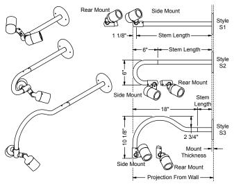
1 1/8" (for Style S1) 6" (for Style S2) 18" (for Style S3) Projection From Wall = Stem Length + Mount Thickness
